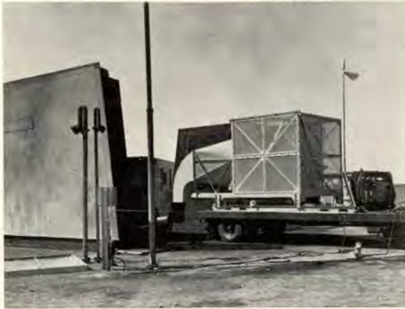
Purge unit provides downward flow of air for cooling and dissipation of gases. Immediate service of unit must be available.
